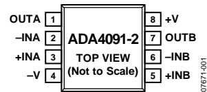
Figure 1. 8-Lead, Narrow-Body SOIC (R-8)
